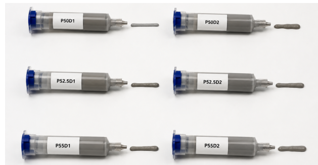
Figure 2. Six prepared hard-PZT inks.
