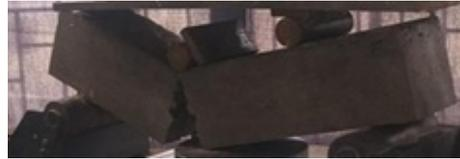
Figure 16. Specimen (Solar dried with PCM) after Flexural Strength test
