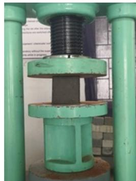
**Figure 7.** GPB under tension split test
