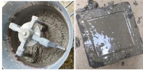
**Figure 3.** Final mixture and mixture poured into mould
