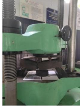
**Figure 9.** GPB under flexural test
