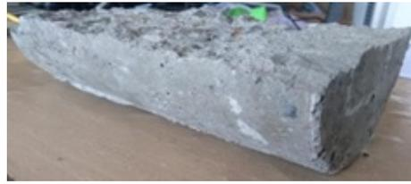
Figure 15. Specimen (Solar dried with PCM) after Compression Strength test
