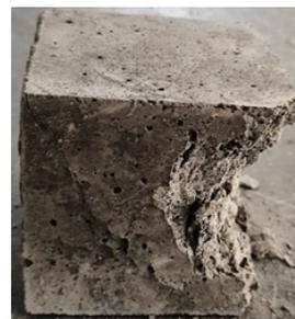
Figure 14. Specimen (Solar dried with PCM) after Tensile Split Strength test
