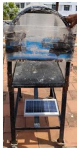
**Figure 1.** Solar dryer
