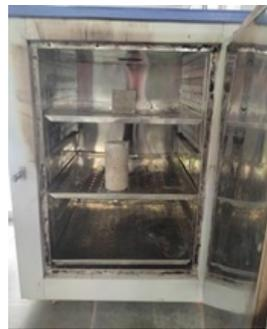
**Figure 5.** Novel GPB (cubic and cylindrical) specimen kept in electric oven
